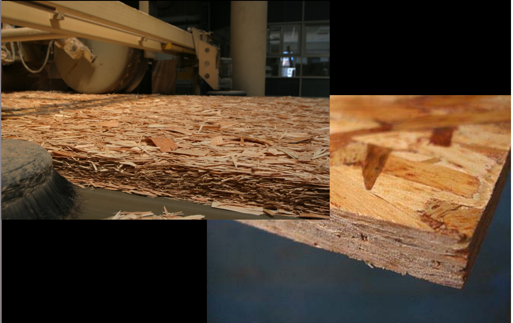
Figure __: The thick pile of carefully sized wood chips is compressed with resin into OSB panels. Credit: wikimedia
