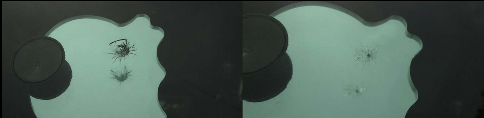
Figure __: Repairing fractured glass can virtually eliminate the apparent damage, but the technology does not have a long history. Credit: mswindshield.com
